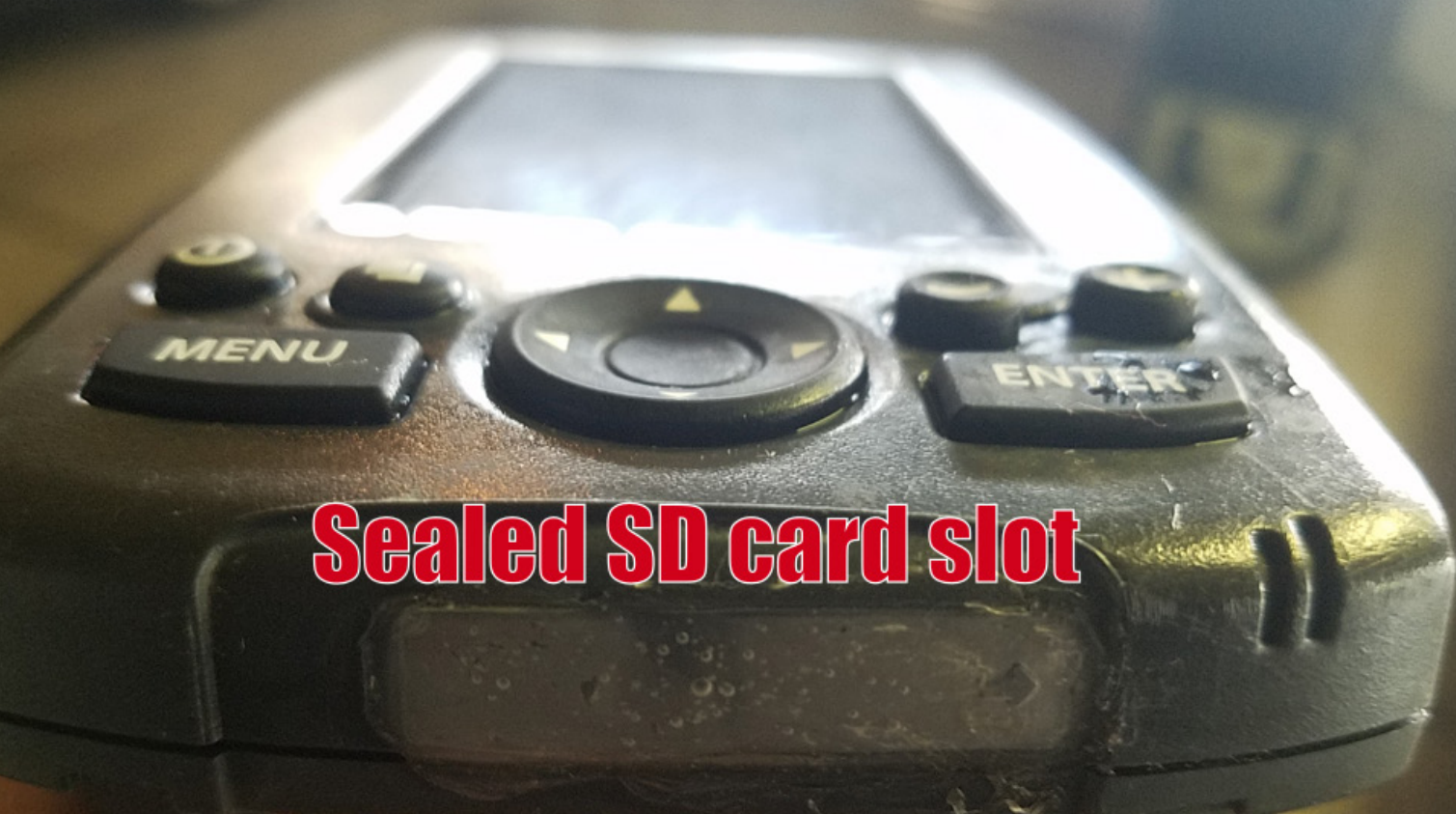
(SD Card Slot Corrosion is why most Lowrance Units Fail)
